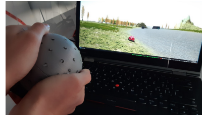
Fig. 9. A user enjoying the racing game demo. Directional haptic feedback is given when the car crashes into an obstacle to inform the user where the crash occurred (relative to the car). The pin force scales with the impact velocity.
