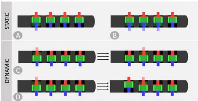
**Figure 4.** MagTics affords two main class of actuation modes. *Static*. (A) Single Pin: an individual taxel moves from up (red) to down (blue transparency). (B) Numeric: consecutive taxels move from up to down to render the number three. *Dynamic*. (C) Single Pin Directional: following one direction, a taxel moves from down to up, to eventually return to its original position. (D) Numeric Directional: following one direction, a taxel moves from down to up and eventually keeps its position.
