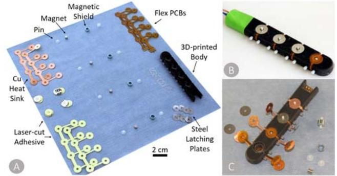
**Figure 3. MagTics' components and assembly.** A) All elements prior to assembly. B) MagTics with each taxel at a different assembly state. The PCB is routed along the bottom of the device (thus providing the bottom coils), and wrapped around the sides of the device, bringing the top coil into position. A steel latching plate is bonded on the coils, followed by a thin copper heat sink. C) A completed device, with the rightmost taxel lacking a latching plate to reveal the coils.
