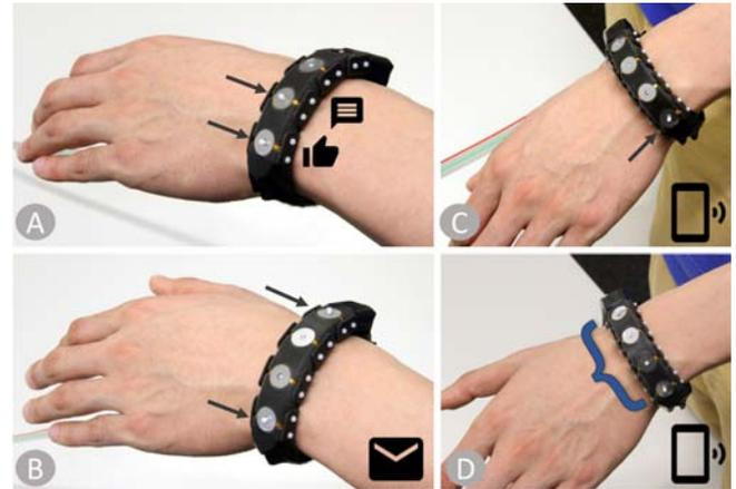
**Figure 5.** Our wristband prototype with bi-directional actuation. (A) Individual taxels are actuated to signal application notifications (here a social network notification and a text message). (B) A U-shaped pattern notifies of new email. (C–D) In the event of an incoming call, the Numeric Directional mode is actuated (C, start and D, end of notification).
