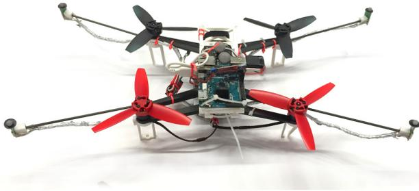
Fig. 3. **Quadrotor with UWB units.**
